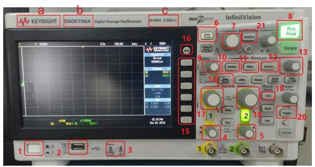
The scope has two input channel where we provide the signal to be measured, the DSO can plot and measure two signals simultaneously. The other input is for external trigger purpose.
