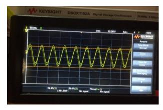
**High-Resolution Mode**: High-resolution mode is another form of averaging. However, instead of waveform-to-waveform averaging, it is point-to-point averaging. Essentially, the ADC oversamples the signal and averages neighboring points together. This mode uses a real-time boxcar averaging algorithm that helps reduce random noise. It also can yield a higher number of bits of resolution.
