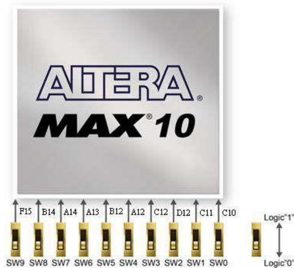
Connections between the slide switches and MAX 10 FPGA
