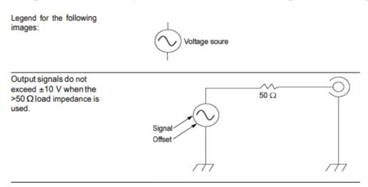
A change to the load impedance (L) will affect the output window (maximum and minimum levels) for a sine waveform as follows.
