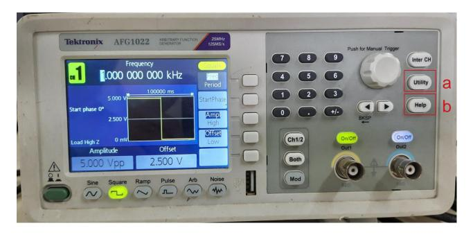
a. The Utility option provide the access to Display Setup, Counter Setup etc. The front menu of the utility is illustrated below
