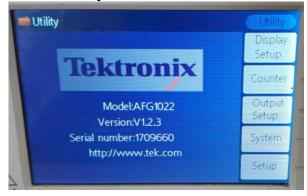
Display Setup: user have access to very the brightness of the screen and can change the screen saver.
