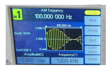
a. The first menu from top right is Mod, user can generate different modulations Like amplitude modulation, frequency modulation etc. Here user can set the carrier and modulating signal parameters. The below image represents the menu of Mod window.
